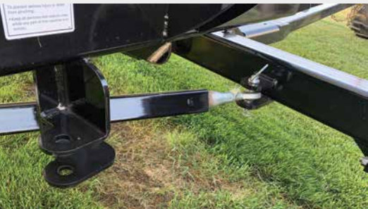
Crossover Tube Assembly Shown In Articulation Mode
