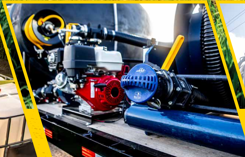
(Unit Shown - 48' trailer, dual 3210 tanks, EZHR300 hose reel, AS-300 pump, dual 60 inductors, 100 rinse system)
