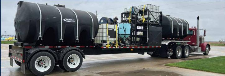
The Quad Tote Rack system conserves deck space and allows four chemical shuttle tanks to be transported in the space that normally can only hold two. Available with a center locker system with four shelves to transport and store hand-pour products. The locker has capacity to hold up to 32, 2.5-gallon jugs with an adjustable backstop and retrieval system.
