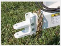
Adjustable Hitch The hitch has an adjustable clevis to accommodate a wider range of drawbar heights, and allows for leveling of the spreader.
