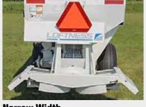
**Narrow Width** With a hopper width of 48.7 inches and tire width of only 50.1 inches, the OS170 can operate efficiently in some of the narrowest spaced plantings.
