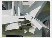
**Consistent Spread Pattern** Dual stainless steel spinners produce a consistent spread pattern up to 25 feet wide on the standard model. A 40-foot spread width is optional.
