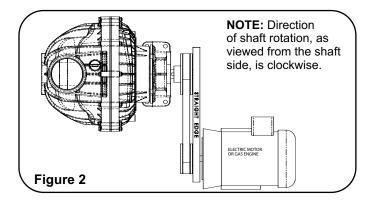
To figure proper diameter of pump pulley, multiply motor/engine rpm by diameter of the motor/engine pulley and divide that figure by desired pump speed.
