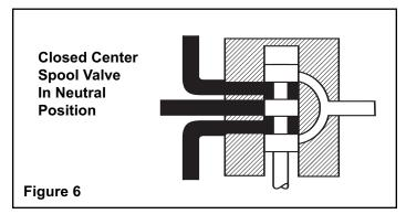
The Closed Center Valve (See Figure 6) is used with variable displacement pumps. The flow is completely shut off in the neutral position, causing the pump stroke to adjust to zero flow. The flow stops, but the pump maintains a static pressure up to the valve.
