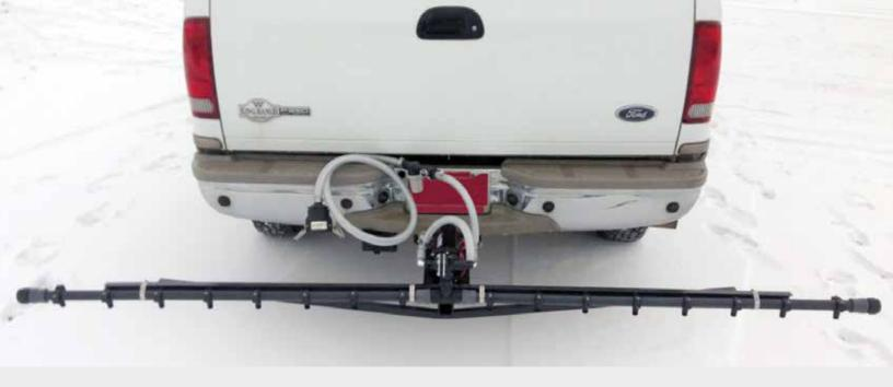
Pre-Treat and Deicer Spray Boom quickly and conveniently attaches to any 2" receiver hitch.
