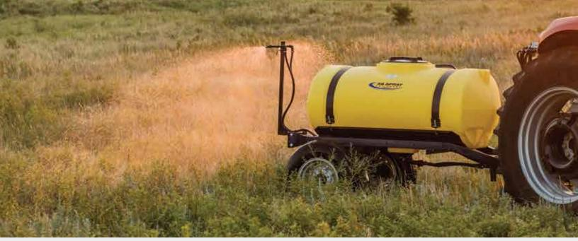
Boomless sprayers are ideal for spraying extremely rough terrain, such as range land, that conventional booms may not withstand. Available in 3PT or trailer mount units. Coverage for 24 Ft. to 40 Ft.
