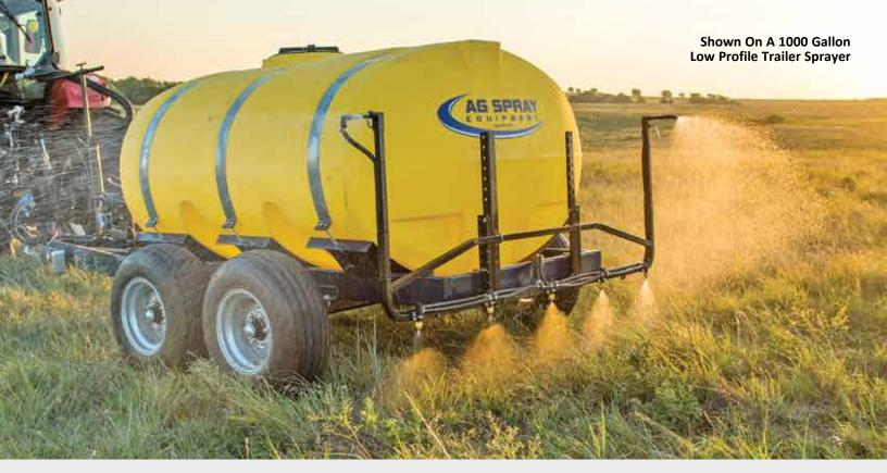
Longhorn boom is an excellent choice for pastures, fence lines, drive lanes, field boundary's and roadside spraying. Utilize the 100" flat fan boom for driveways and crop lanes and extend the spray with the boomless side mounted nozzles to reach out up to 16' each side for a combined 40' coverage.
