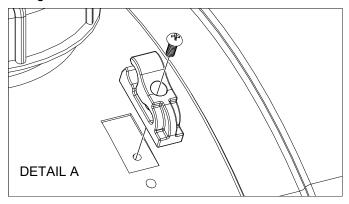
Locate the (2) clips and (2) phillips head screws from the parts bag.
