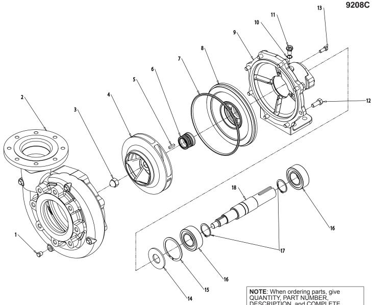
Mechanical Seal Kit #3430-0604 Includes Items 6 & 7 Bearing Kit #3430-0671 Includes Items 14, 15, 16, 17 **NOTE**: When ordering parts, give QUANTITY, PART NUMBER, DESCRIPTION, and COMPLETE MODEL NUMBER. Reference number are used ONLY to identify part in the drawing and are NOT to be used as order numbers.
