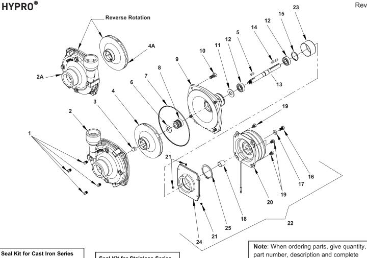
Seal Kit for Cast Iron Series No. 3430-0332 Consists of: (1) Ref. 7 O-ring, (1) Ref. 8 Mechanical Seal, and (1) Ref. 6 Gasket
