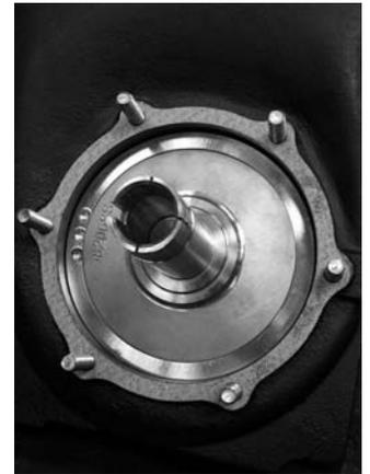
6. Install seal spring assembly on the impeller shaft. Lubricate the shaft and viton portion of the seal with petroleum jelly. Slide onto shaft using your thumbs.
