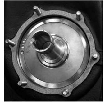
7. Remove the seal assembly (15035) from the wet seal assembly at this time.
